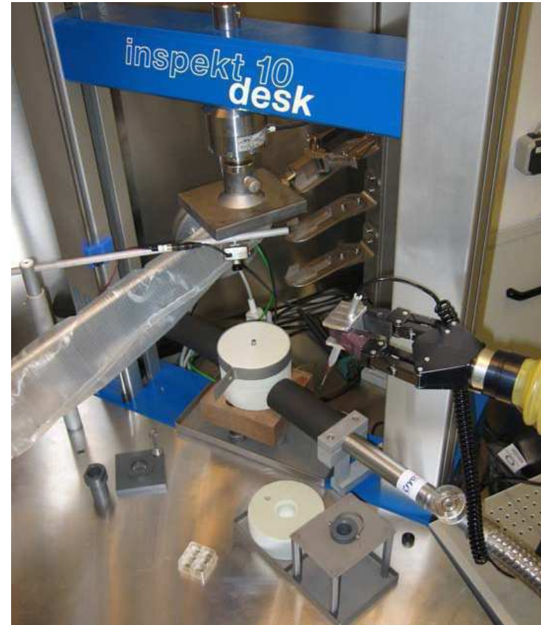
Fig. 2: SPT in a hot cell at FZD. Sample is located within a small temperature chamber ( -185^{\circ}\text{C} - +250^{\circ}\text{C} ). Samples are square plates 10 \times 10 \text{ mm} t=0.5 \text{ mm} . No downholder, larger die d=6.8 \text{ mm} \rightarrow larger plastic volume.
