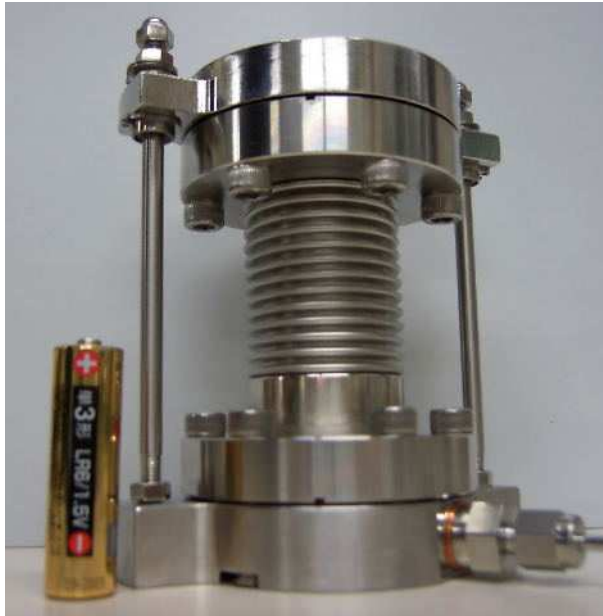
Appearance of developed in-situ SP test apparatus equipped with a gas flow system.
